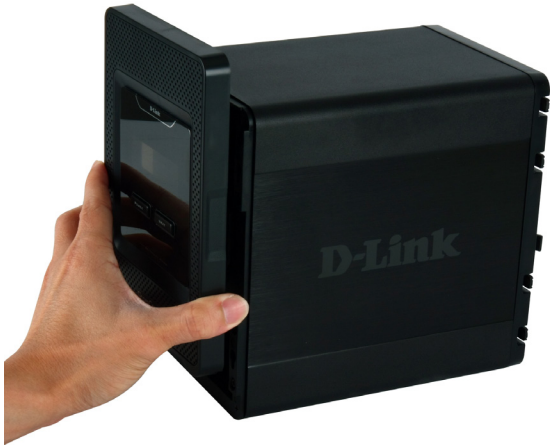
Detach the front cover of the NAS
